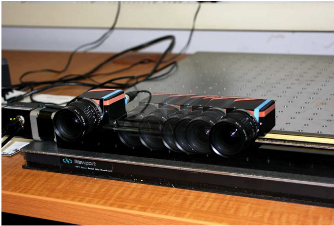
Fig. 7 Our setup to simulate a pushbroom camera. The camera (Prosilica) is mounted on a programmable linear stage. The accuracy of the stage is in the 100th of millimeter.
